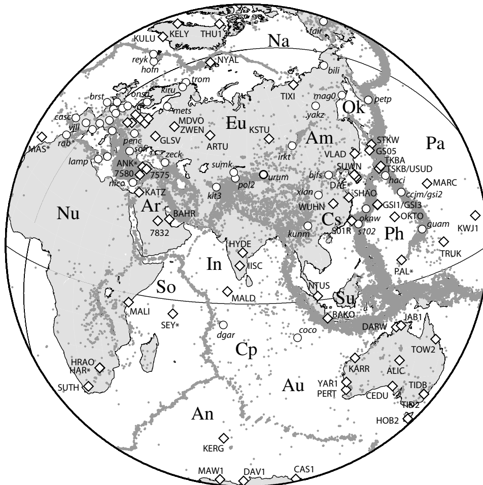
Figure 5. Lambert azimuthal equal-area projection showing all space geodetic site locations used in this study for the area around the Indian Ocean. Earthquake epicenters (magnitude >4.5 , depth <50 km, between 1973 and 2000) suggest plate boundaries. Sites labeled with diamonds and upper case letters are assumed to lie on the rigid plate interior and are used to define the plate's angular velocity (Table 2). Sites labeled with circles and lowercase letters are not used in the rigid plate definition (Table 2). See Table 1 for plate abbreviations, except Cp, Capricorn. For clarity, site names in some areas have been omitted, e.g., Europe.
