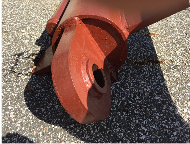
Figure 7 (top) main buoy; (base) close-up of attachment point, which connects with the seafloor ballast through a large shackle (Figure 8).
