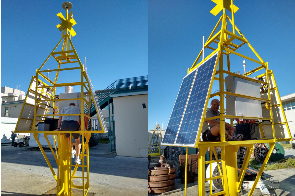
Figure 3. Buoy superstructure. This part of the buoy is above the waterline, and is designed to be lightweight and with low cross-section area to minimize wind stress. The GPS and associated electronics are mounted inside this framework (grey box; see Figure 3 for close-up) while the solar panel is mounted externally. The GPS antenna is mounted at the top (left-hand figure).
