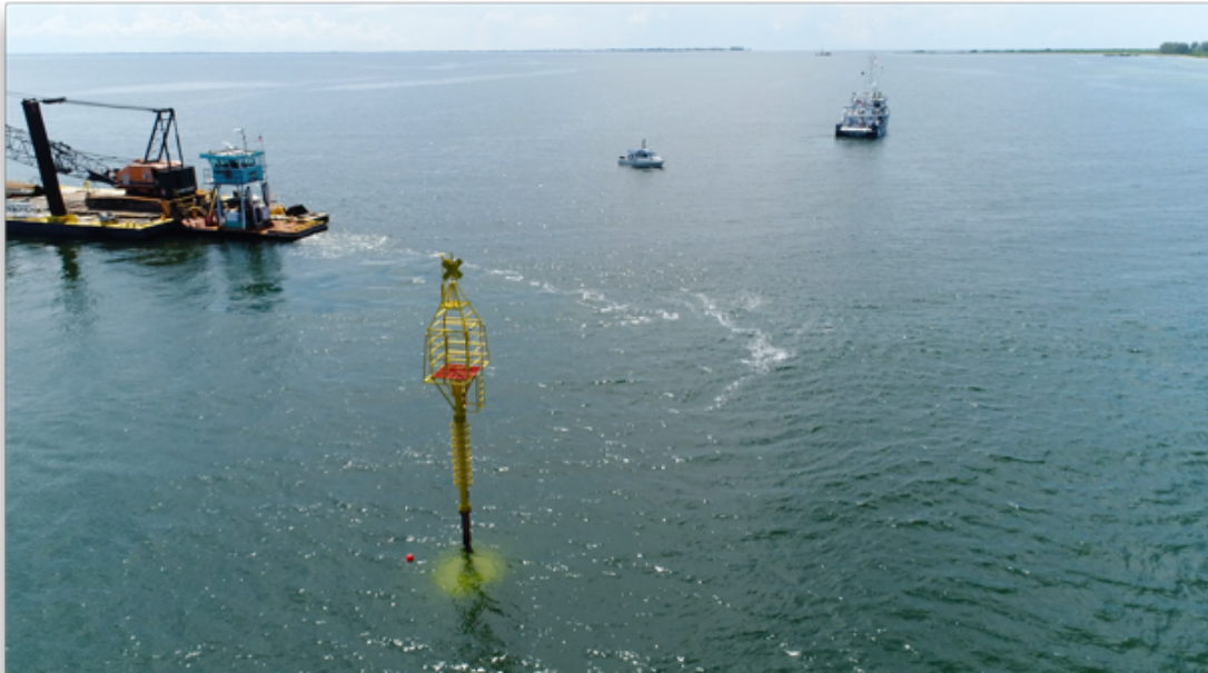
Figure 15. Buoy immediately after deployment, prior to installation of electronics. Note top of float (yellow) approximately 2 meters below the surface.
