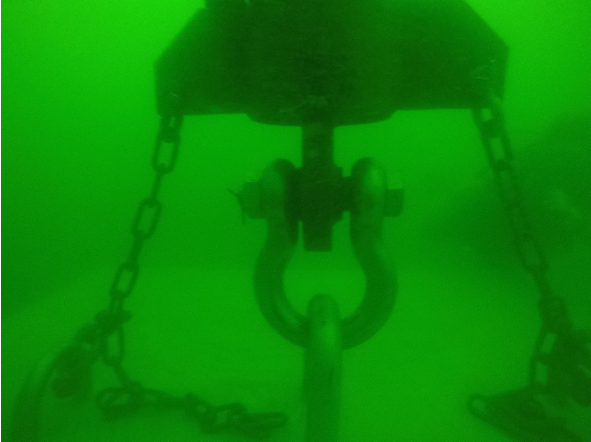
Figure 8b. Shackle after deployment on the sea floor, connected to ballast.
