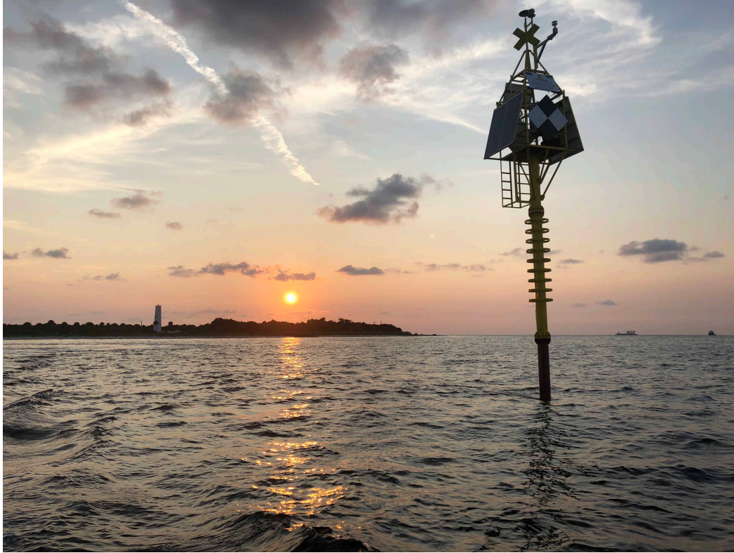
Figure 17. The buoy with electronics, solar panels and signage installed. Egmont Key is in the background. Note tilt of buoy, reflecting strong tidal current.
