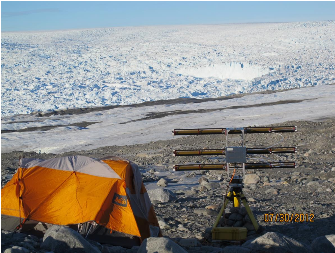
Figure 8.10a. The calving front at Jakobshavn Isbrae during summer, 2012. An instrument for measuring ice velocity is visible in the foreground, along with a small tent to shelter the operators (the author and graduate student Denis Voytenko) from the wind. The arcuate ice front is approximately 150 meters high, and its center is 5 km away, near the upper right hand side of this photo. The Greenland ice sheet is in the background and to the right of the ice front. Jakobshavn's ice-filled fjord is at the center-left, below the front. Ice motion is mainly from right to left. Photo by the author.
