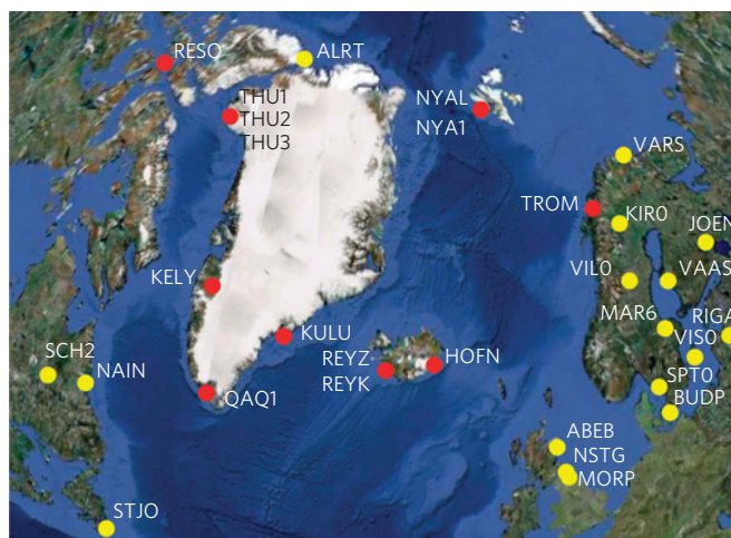
Figure 1 | Location of GPS sites used in this study. The red circles indicate sites with acceleration 0.5 \text{ mm yr}^{-2} or greater; the yellow circles indicate acceleration less than this value.
